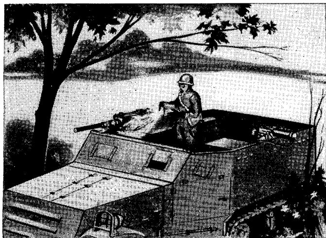
FIGURE 44.—Do not pour lime slurry on interior of vehicles, weapons, instruments or fabric equipment. It will corrode or destroy them.
